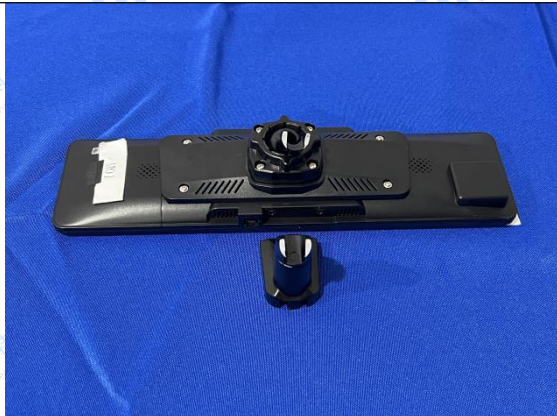
Fig.6 Appearance inspection after test (The front impact bracket has fractured)
