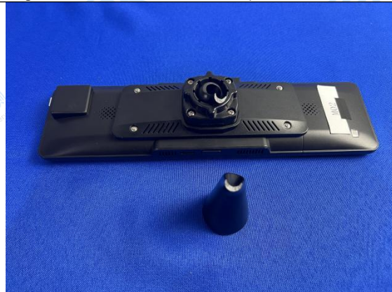
Fig.7 Appearance inspection after test (The 45-degree impact bracket has fractured.)
