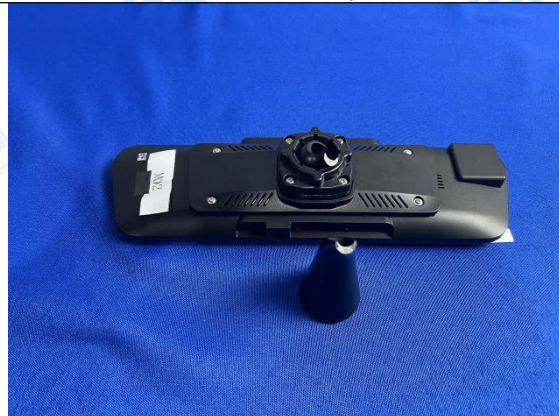
Fig.7 Appearance inspection after test (The 45-degree angle impact caused the support to break.)
