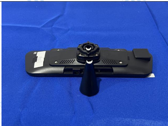
Fig.6 Appearance inspection after test (Frontal impact caused the support to break)
